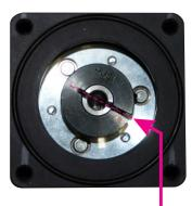
The inner and outer slit is aligned as they should.
